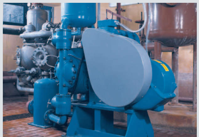
Tested, stable design. ABEL CM piston diaphragm pump for filter press feed
